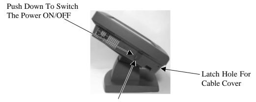
Slide Switch For Power On/Off Control
